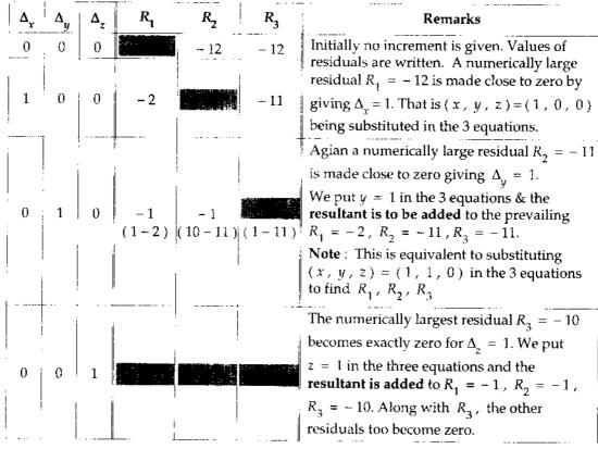
It can be seen that  $R_1$ ,  $R_2$ ,  $R_3$  are all zero and the exact solution of the given system is  $x = \sum \Delta_x = 1 + 0 + 0 = 1$ ;  $y = \sum \Delta_y = 0 + 1 + 0 = 1$ ,  $z = \sum \Delta_z = 0 + 0 + 1 = 1$
